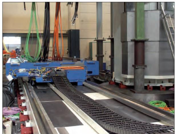
Holding chainflex®-cables in e-chains® for motion-control applications.
