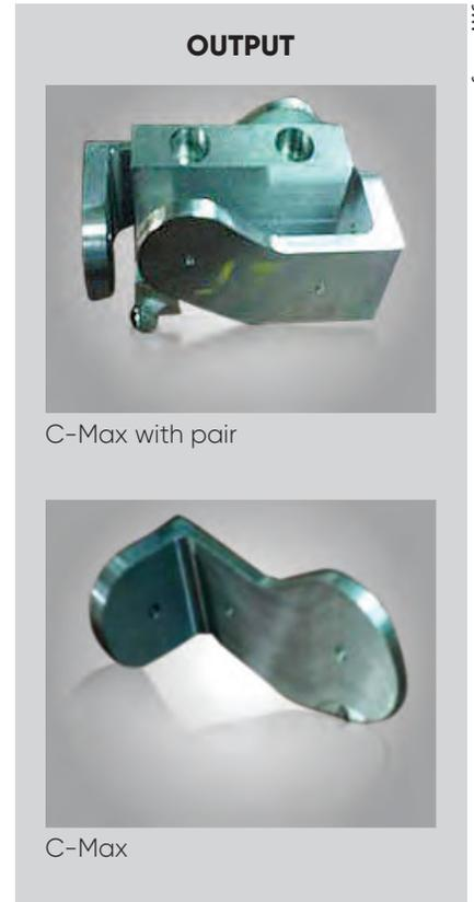
out which ensures vibration-free machining. The CMH400XL – column moving type horizontal machining centre from AMS – incorporates the features. With machining done on the machine, the cycle time was reduced from 20:55 min to 5:35 min, in addition to significant improvements in accuracy and surface finish. **CNC<sup>Plus</sup>**
