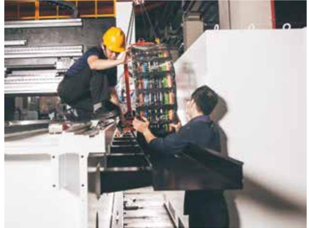
In its robotic machining centres, many companies use fully harnessed energy chain systems from igus. This cuts out many process steps for the manufacturer, reducing assembly time from several weeks to just half a day. Another benefit receives is from a single source and delivered onsite fully-tested for reliability and safety.
